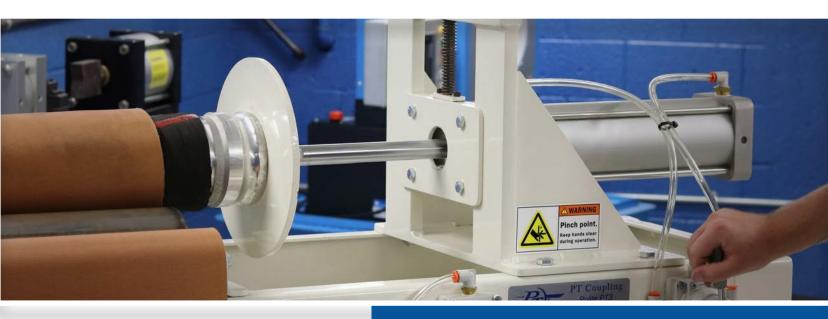
ROLITE PT3 FITTING MASTER is PT's solution for an easy installation and removal of fittings when handling hose assemblies. With pneumatic controls, and manufactured from high quality materials, the Rolite is the simple and cost-effective solution for high production hose assembling.
